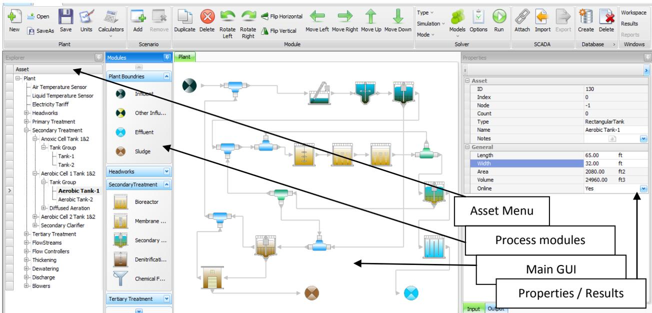
**Figure 1.** Application of Complete Asset Hierarchical Structure to Communicate with Process and Asset Management Models (Screen shows Asset Menu and Modules to the left of GUI, Properties and Results menus on the right).
