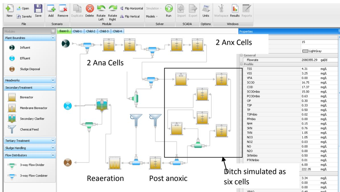
**Figure 4.** Plant has 2 anaerobic cells receiving RAS, two anoxic cells receiving nitrate recycle from ditch, ditch (simulated as follows: aerobic with Eimco mechanical aerator, anoxic, anoxic, aerobic with Eimco mechanical aerator, anoxic, anoxic), post anoxic with optional glycerol feed, reaeration with optional Aluminum Hydroxide feed, Clarifier.
