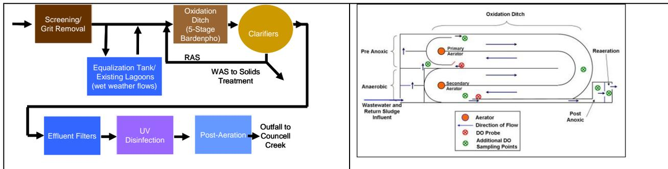
**Figure 3.** Layout of Easton Plant, Maryland, USA. 16,000 m<sup>3</sup>/d plant operating at Average flow of 8100 m<sup>3</sup>/d in 2009
