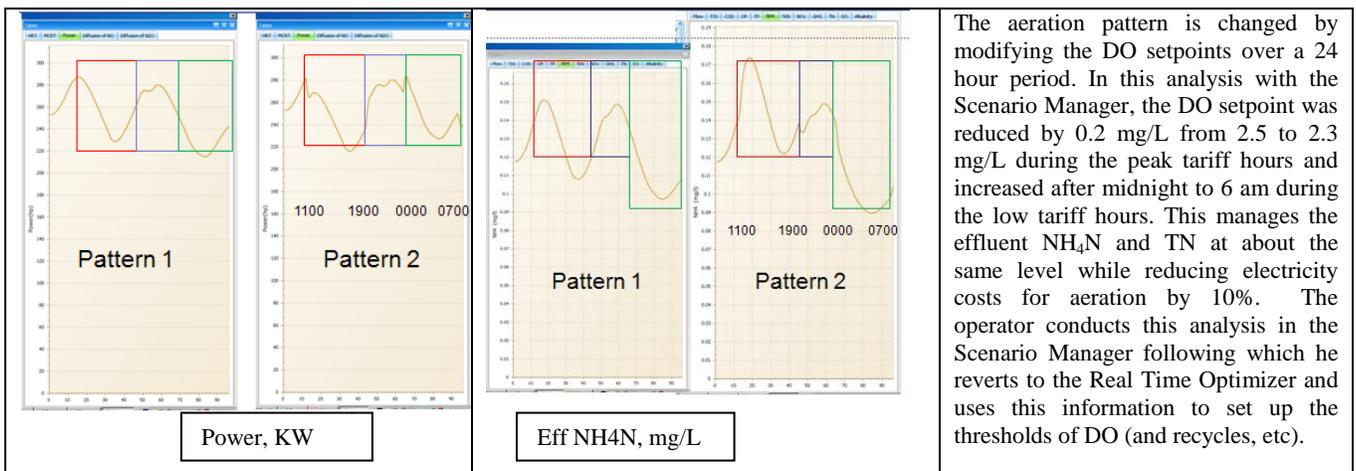
**Figure 8.** Optimizing performance through Scenario manager to achieve same levels of nutrient removal at lower costs
