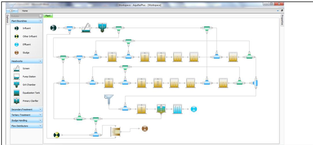
**Figure 7.** Complete Layout as used in Westminster, MD. The North and South Trains have different types of diffusers.
